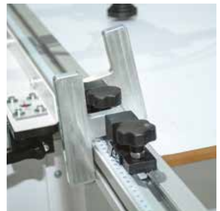
Bi-directional flip stopper both LH and RH lateral fence
