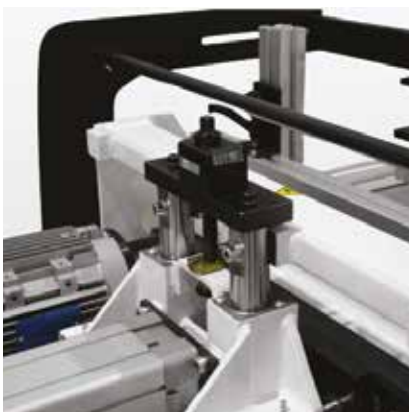
Z1 Height adjustments with position indicator
